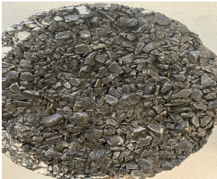
Pictured Above: Core of Mat Seal w/ Double Seal
